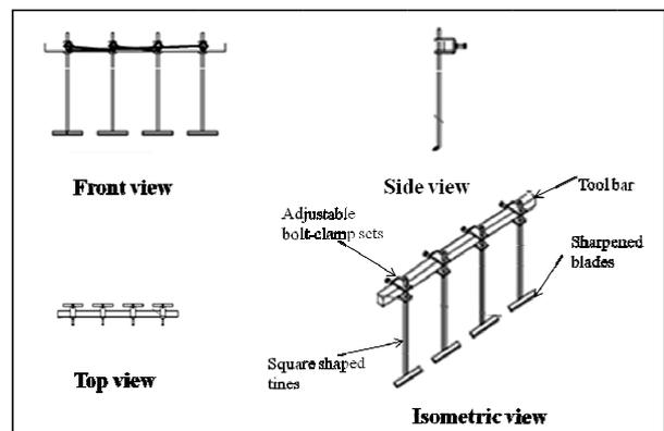
Fig. 1: Schematic diagram of the developed mechanical weeder
