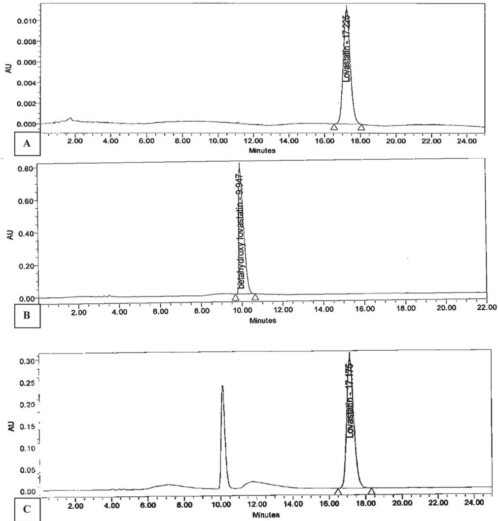
Fig. 2: Reverse Phase HPLC analysis of Lovastatin
