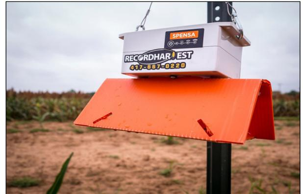
Spensa sentinel open ups the way for identification and counting of number of insects that attracted inside the pheromone based adhesive trap by utilizing deep learning algorithms in the cloud system.
