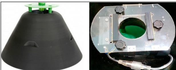
Black pyramidal trap which contains the aggregation pheromones along with optical sensor sense adult pests that enter the trap and count the number of pests as well. It also has the facility to measure the environmental parameters. This collected data are
