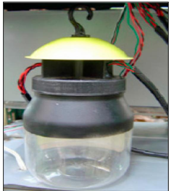
Liao *et al.* (2012) develops the monitoring system to improve the above-mentioned method. It consists of Wireless Monitoring Node (WMN), Remote Sensing Information Gateway (RSIG) and Host Control Platform (HCP). Information was collected by WMN and it is passed to Remote sensing information gateway and finally reach the Host control platform for processing. The server classifies the data and deliver various events i.e., A normal status event, A pest outbreak event and Sensor fault event.
