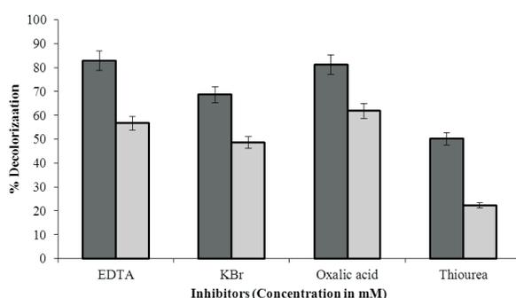
**Figure 3(c): Effect of inhibitors on decolorization of Reactive Black B (■ 1mM, - 2.5mM of inhibitors)**
