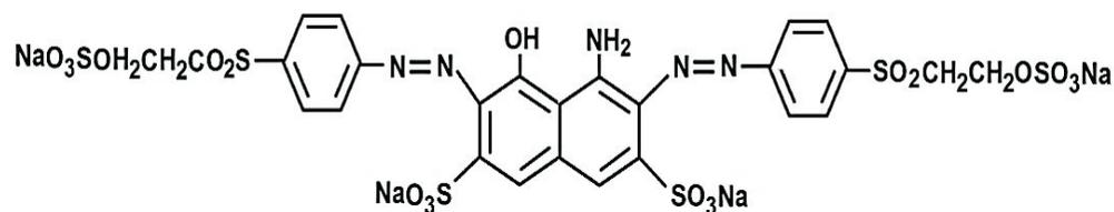
Figure 1: Chemical structure of sulfonated di-azo dye Reactive Black B
