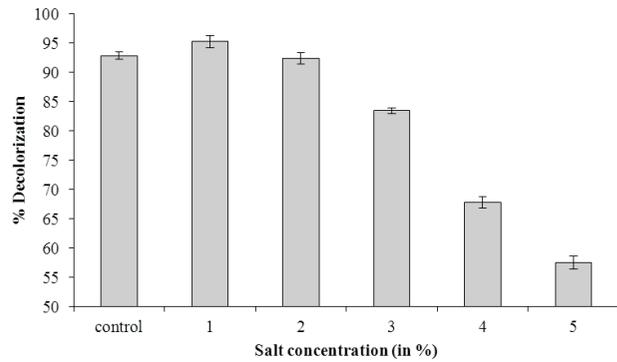
**Figure 3(a):** Effect of salt concentration on decolorization of Reactive Black B
