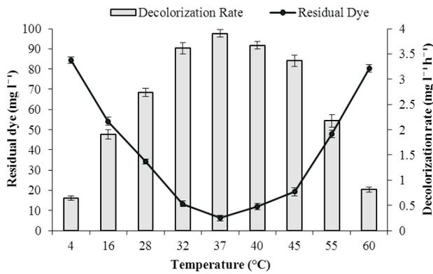
**Figure 2(b):** Effect of temperature (°C) on decolorization of Reactive Black B
