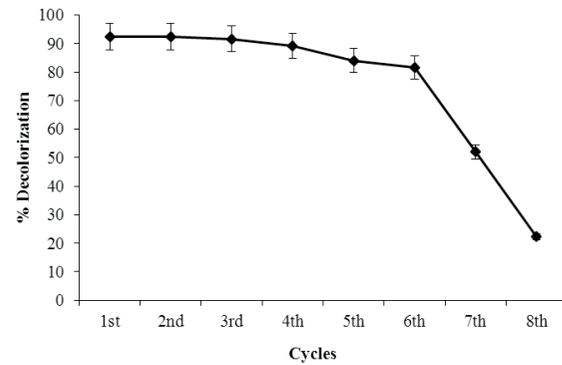
**Figure 2(e):** Effect of split dose addition on decolorization of Reactive Black B
