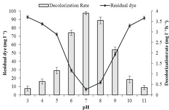
**Figure 2 (c):** Effect of pH on decolorization of Reactive Black B
