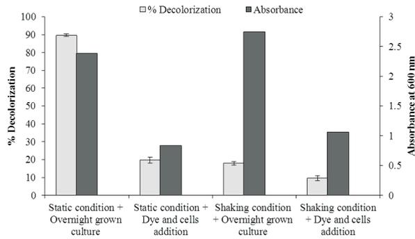
**Figure 2(a):** Effect of mode of incubation (shaking/static) and time of dye addition (after overnight grown culture/dye and cells addition same time) on decolorization of Reactive Black B
