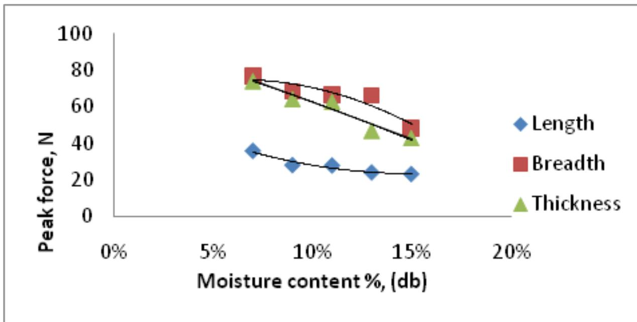
Figure 5. Effect of moisture content on peak rupture force of compression loading of onion seeds along length, breadth of onion seeds at rupture along length, breadth and thickness and thickness
