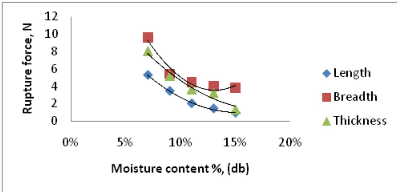
Figure 4. Effect of moisture content on initial rupture force of onion seeds during compression loading along length, onion seeds during compression loading along length, breadth and thickness breadth and thickness
